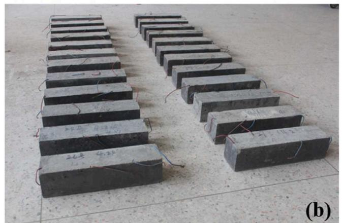
**Fig. 1.** The diagram of (a) the four-electrode method and (b) ECCC samples.
