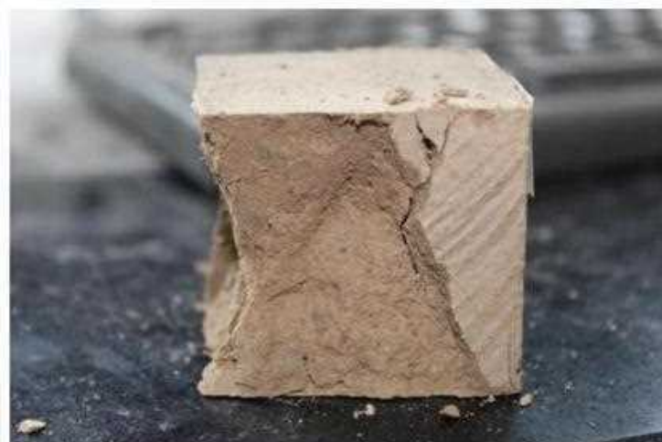
Figure 7. Fracture surface of conventional CSS sample.
