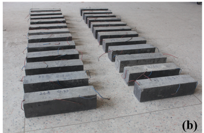
Fig. 1. The diagram of (a) the four-electrode method and (b) ECCC samples.
