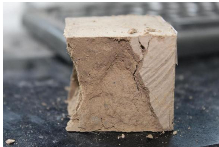
Figure 7. Fracture surface of conventional CSS sample.
